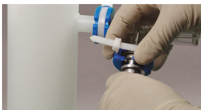
Insert cable tie end and slide clamp closed
