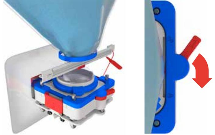
The red rear toggle, marked number 1 must be fully turned to release the interlocks and secure the parts together.
