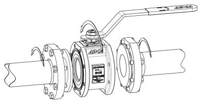
Loose body flanges make it possible to install the valve without aligning of the welded end connections. After installation the valve can rotate on 360° for the desired orientation.
